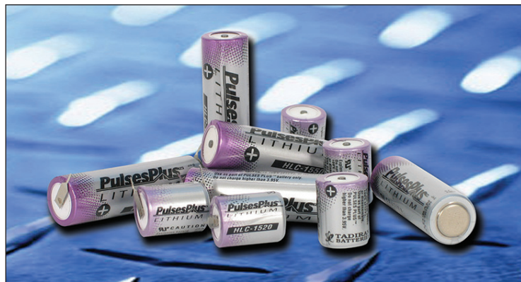
Figure 2. Bobbin-type \text{LiSOCl}_2 batteries can be combined with a patented hybrid layer capacitor (HLC) to offer up to 40-year operating life while providing high pulses to power two-way wireless communications.
