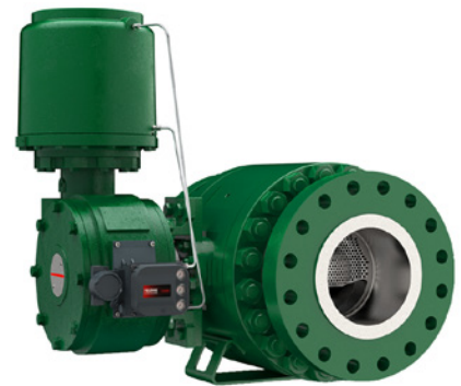
Figure 5. A 900-pound full-bore throttling valve ( Fisher V280 shown) is commonly used in CO 2 pipeline applications. Attenuators for liquid and vapor service may be required for applications with high pressure drops.
