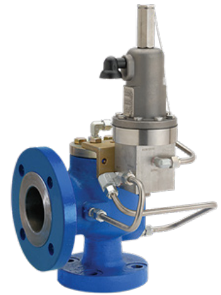
Figure 5. Direct spring pressure release valves (PRVs) can cause emissions, flaring, and product loss. The recommendation is to upgrade to pilot operated PRVs (shown,) which have more precise pressure handling. Courtesy: Emerson
